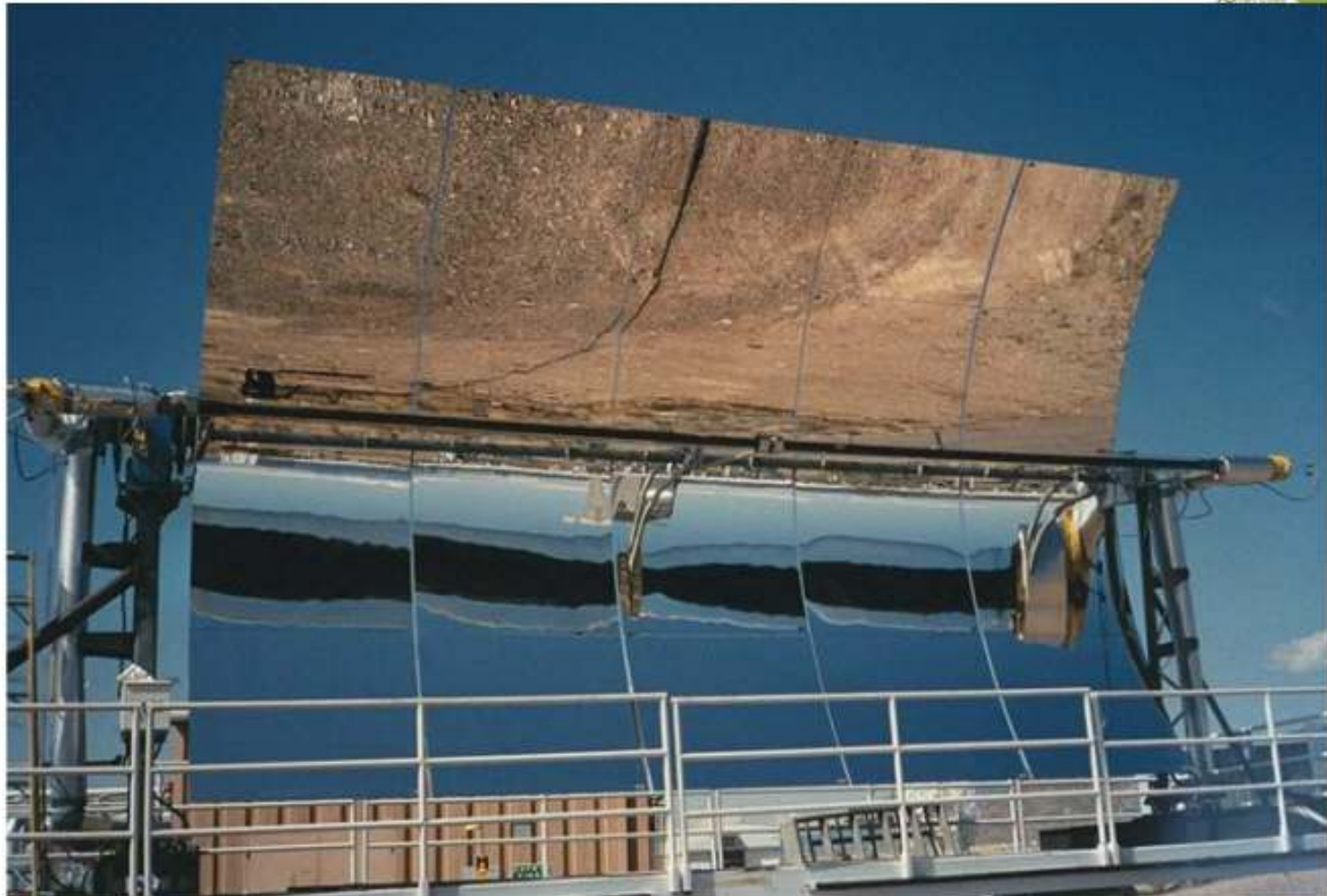
Parabolic trough solar collector system
